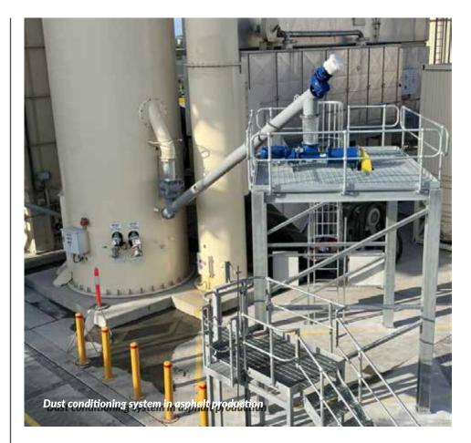
A TOREX<sup>®</sup> Drop-through Rotary Valve as a fundamental component ensures efficient and precise material flow, facilitating the overall functionality of the system.
